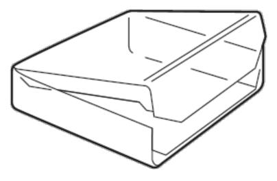
Inspect the protective case for cracks, chips, distortion, or other signs of damage. If the case is damaged the cartridge may be damaged as well.
