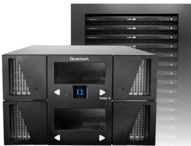
Lattus provides a highly scalable archive repository using object storage technology to provide very high-capacity storage while protecting data by spreading it across many different disk spindles and, optionally, multiple locations.
